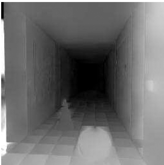
Figure 16: Disparity map obtained through kz2 + stereo-Flow.
