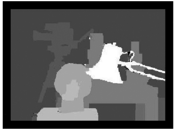
Figure 3: Disparity map obtained through kz2.
