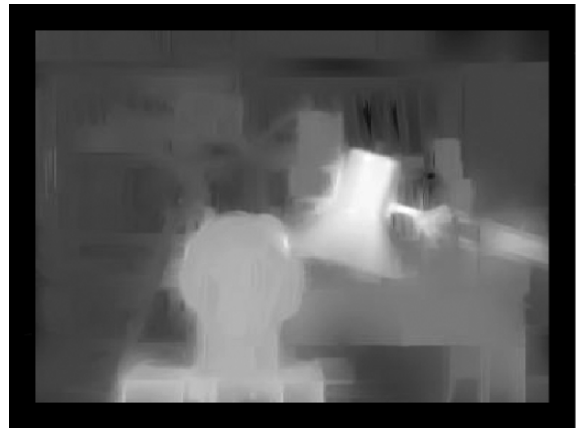
Figure 4: Disparity map obtained through correlation + stereoFlow (using a 21x21 correlation window).
