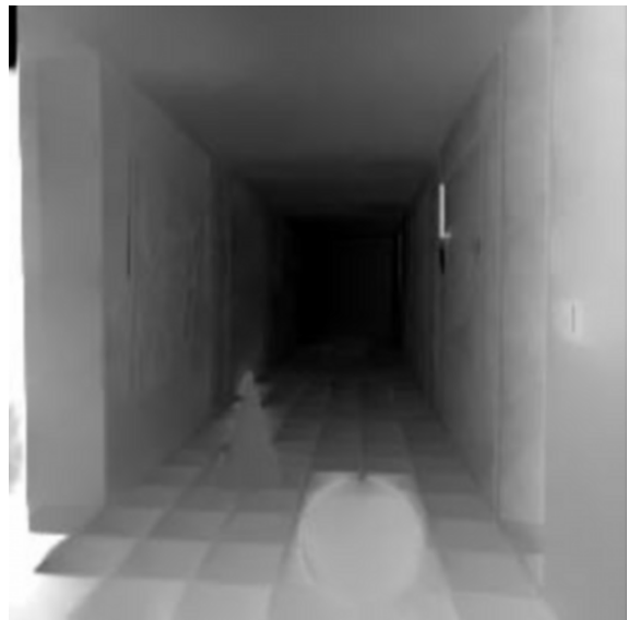
Figure 15: Disparity map obtained through correlation + stereoFlow.
